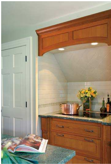
(Above) Utilizing a nook under the staircase, the cooking grotto houses storage for pots and pans, and two pull-out spice units. The induction cooktop is vented via a downdraft unit.
